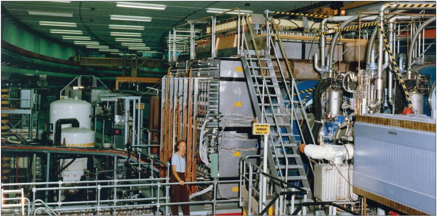
A view of the Axial Field Spectrometer – the last large experiment at the ISR. The horizontal top and vertical outer arrays of the uranium-scintillator hadron calorimeter are clear to be seen, with the blue cylindrical pole piece of the magnet just visible. The pipes that are visible in front of the pole piece are cryogenic feed pipes for the superconducting low-beta quadrupoles.
