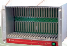
VME8010/VME8011 Low Cost: 21 slot, VME64, integrated or removable Power Supply, integrated Fan Unit.
